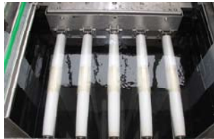
Water tank: Upper rollers
